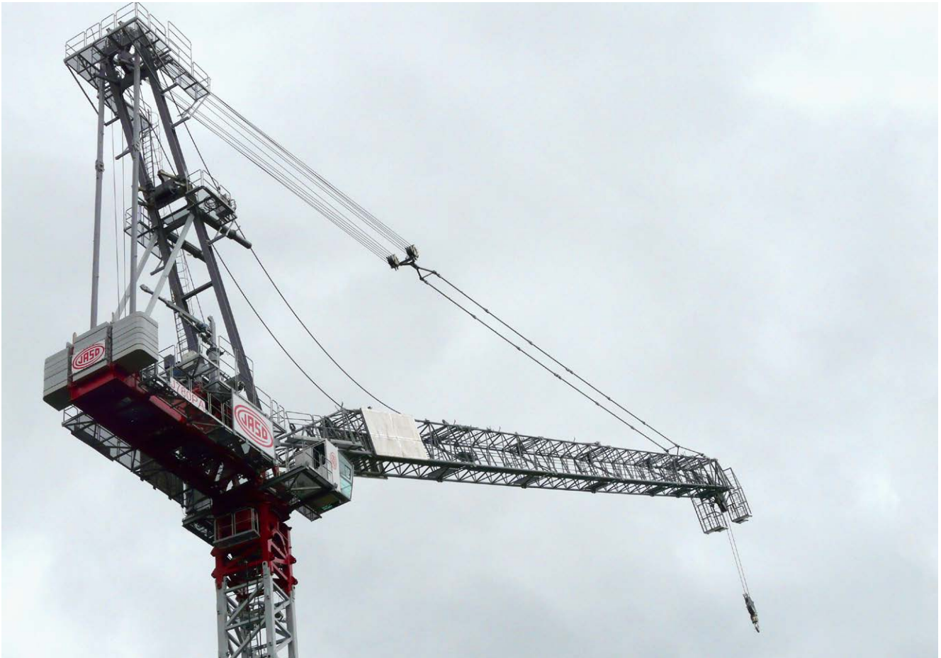
the JASO J780PA. CASAR Doublefit is used as the hoist cable, CASAR Parafit is used as the boom adjustment cable.
